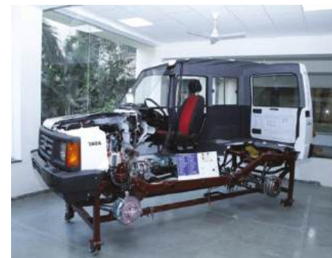
Cut Section of TATA SUMO Vehicle
